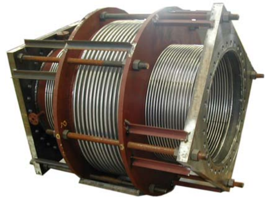
24" In-line Pressure Balanced Expansion Joints designed for 175 PSIG and 610 °F for a petrochemical plant in Venezuela. The bellows are composed of Inco 625 LCF material and the flanges and liners are constructed from SA516 Grade 70 material.
