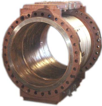
24" dia. Single Hinged Expansion Joints designed for 170 PSIG and 580 °F for a water facility in Pennsylvania
