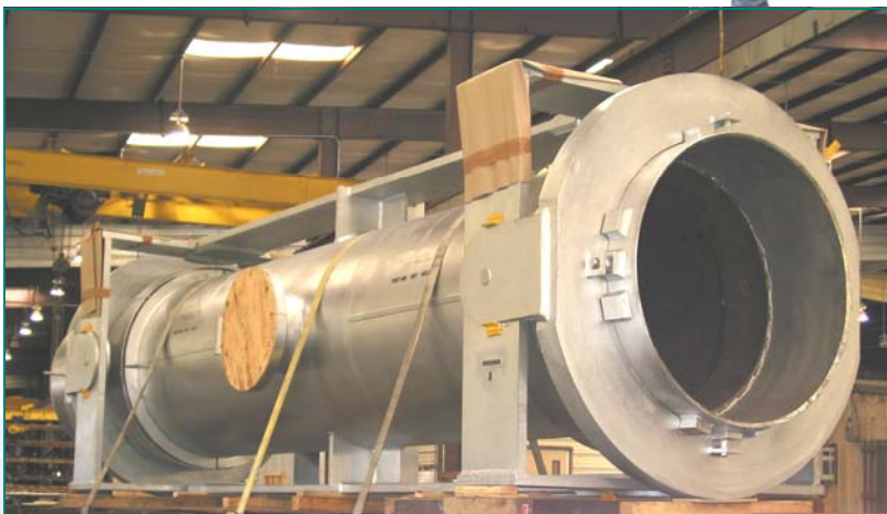
55" O.D. Double Gimbal Universal Expansion Joint for an FCC Unit. The expansion joint is equipped with floating rings and Inco 625 LCF bellows. It is designed for 50 PSIG and 1075 °F.
