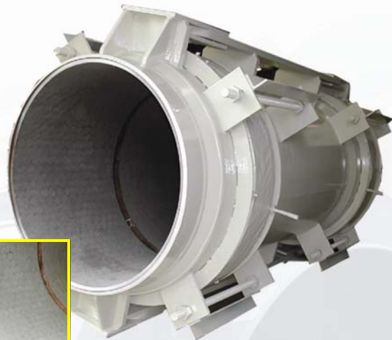
44" Universal Refractory Lined Expansion Joints designed for 30 PSIG and 1400 °F with Inco 625 LCF bellows and a 4" thk refractory lining per UOP specifications
