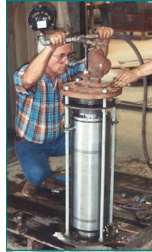
Hydro-testing being performed on a 6" Slip Type Expansion Joint
