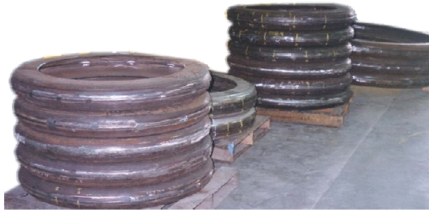
44" thick wall SA516-70 flanged and flued Expansion Joints
