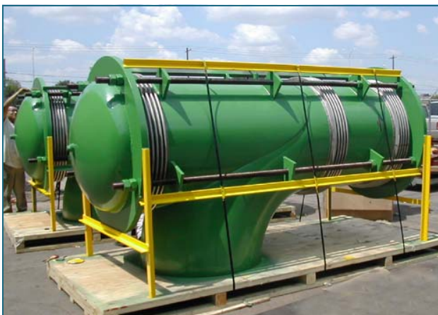
Elbow Pressure-Balanced Expansion Joints designed for 150 PSIG and 450 °F to allow lateral and axial movements in a 42" steam line
