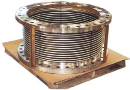
30" dia. Expansion Joint, with 2-plies 321SS bellows, designed for 50 PSIG and 650 °F
