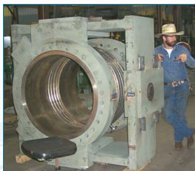
36" Gimbal Expansion Joint after completion
