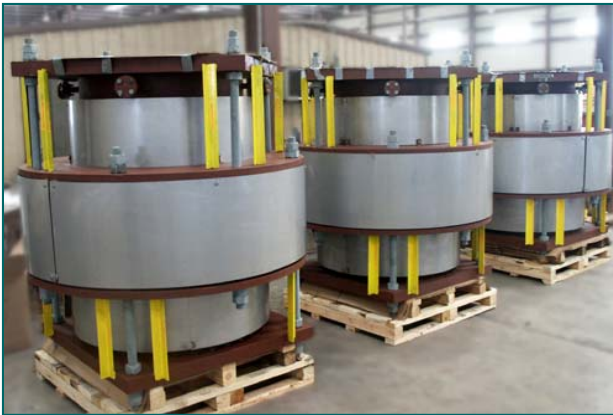
24" In-line Pressure Balanced Expansion Joints designed for 175 PSIG and 610 °F for a petrochemical plant in Venezuela. The bellows are composed of Inco 625 LCF material and the flanges and liners are constructed from SA516 Grade 70 material.
