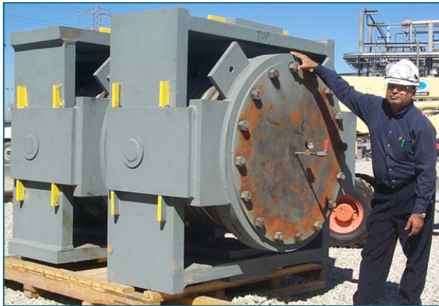
36" dia. Single Gimbal Expansion Joint, with testable Inco 625 bellows, SA516-70 gimbal rings, designed for 680 PSIG and 270 °F
