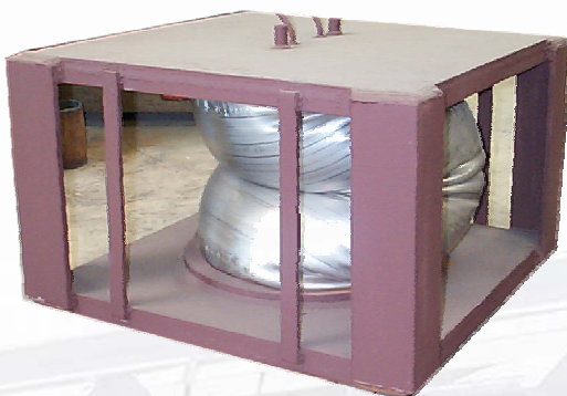
Burst Test on a 20" Bellows as per US Army specifications
