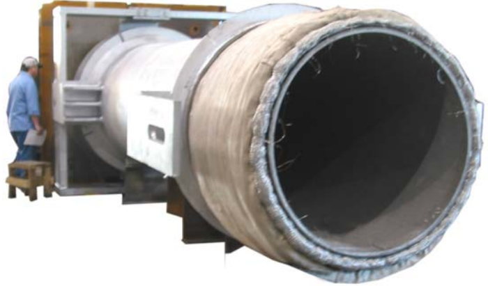
In Process: 56" O.D. Gimbal Hinged Refractory Lined Universal Expansion Joint for a CAT Cracker Application, designed for 57 PSIG and 1300 °F
