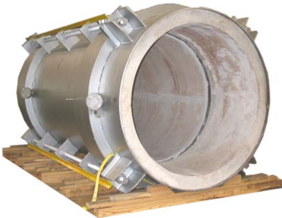
70" Tied Universal Expansion Joint with a 4" thick Refractory Lining per UOP specifications, designed for 51 PSIG and 1460 °F
