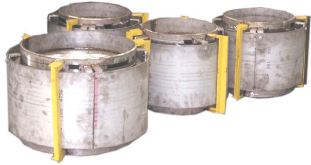
24" dia. Single Expansion Joint, with 321SS bellows, liner and cover, designed for 50 PSIG and 651 °F
