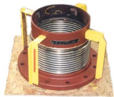
12" dia. Single Expansion Joint, with 304SS bellows, SA 105 150# RFSO and C/S weld ends.
