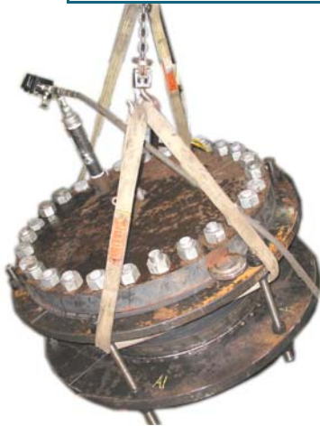
Hydro test on a 30" Rubber Expansion Joint designed for 150 PSIG and 221 °F
