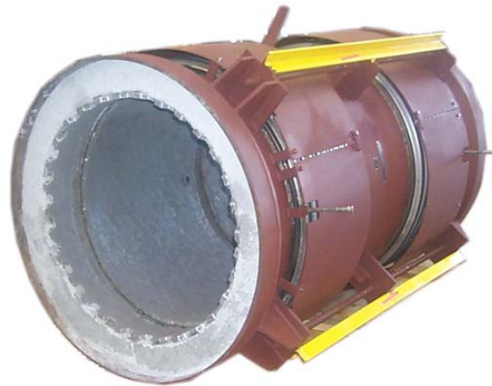
44" Universal Refractory Lined Expansion Joints designed for 30 PSIG and 1400 °F with Inco 625 LCF bellows and a 4" thk refractory lining per UOP specifications
