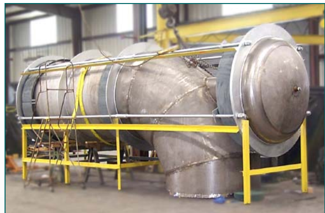
72" Universal Pressure Balanced Expansion Joint designed for 30 PSIG/full vacuum and 200 °F
