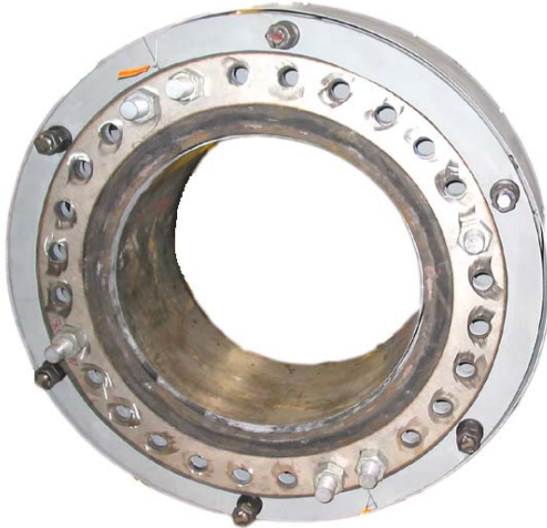
30" dia. Rubber Expansion Joint, with EPDM reinforced tube and cover, telescoping linear A516-70 flanges, designed for 150 PSIG and 221 °F
