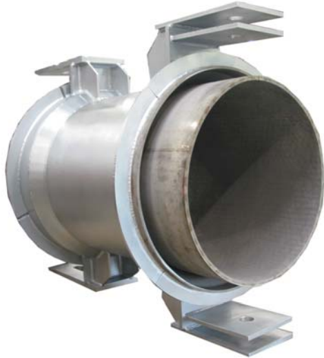
In Process: 55" O.D. Gimbal Hinged Refractory Lined Universal Expansion Joint for a FCC Unit, designed for 60 PSIG and 1020 °F
