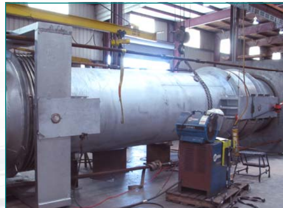
Pneumatic and Vacuum test between piles at 15 PSIG/14 PSIG for a 56" O.D. Gimbal Hinged Refractory Lined Universal Expansion Joint
