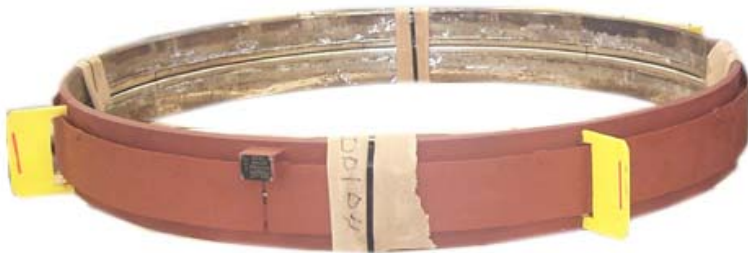
92" I.D. Toroidal Bellows Expansion Joint designed for 400 PSIG and 500 °F
